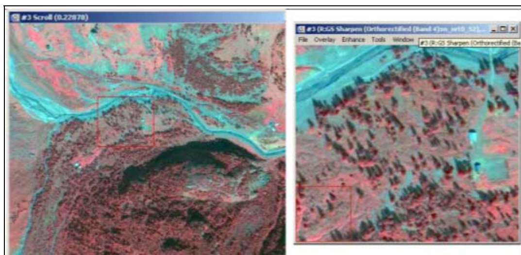
Figure 5: Fused image ("pan-sharpened")
